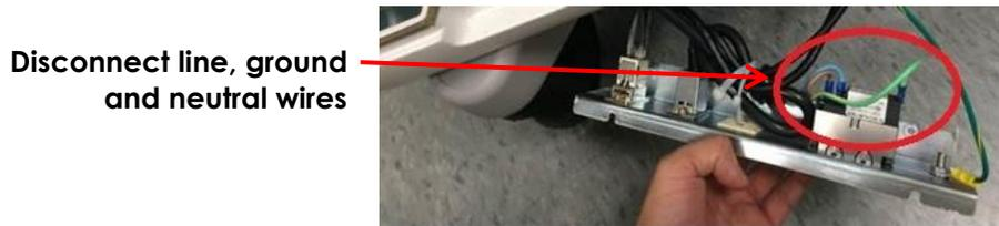
Figure 117: Line Filter Cable Wires
