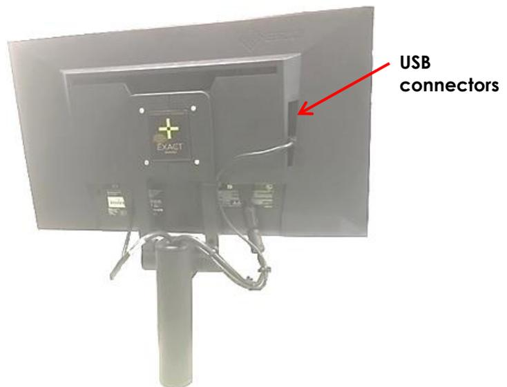
Figure 38: USB Connectors on the Rear of the Monitor (ExactVu 2.6/2.9 hardware versions)
