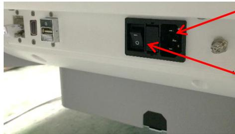
**ExactVu system power cable receptacle****Main power switch (in the OFF position)****Figure 15: ExactVu System Power****To disconnect power from the ExactVu system:**
