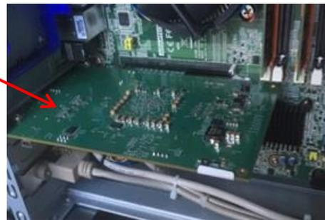
Figure 82: Beamformer Control Board (BCB)
