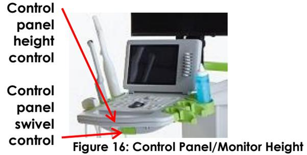
Figure 16: Control Panel/Monitor Height
