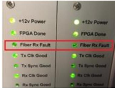
**Figure 135: Fiber Rx Fault LEDs on the Channel Boards**
