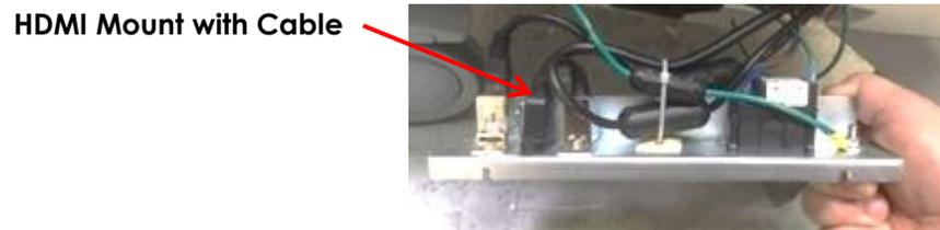
Figure 78: HDMI Mount with Cable
