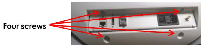
Figure 77: Screws Securing IO Plate Assembly
