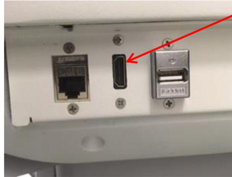
**Figure 18: Second Monitor Output (HDMI) Connector**
