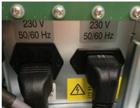
**Figure 143: Card Cage Power Cable Connections**
