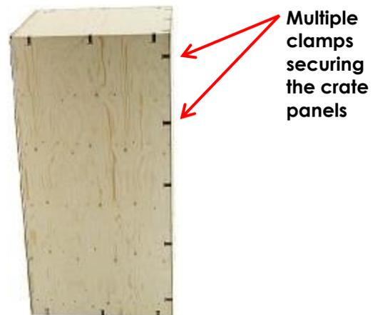
Figure 8: Clamps Securing Crate Panel
