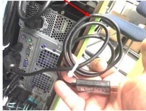
Figure 76: Display Port to HDMI Adapter Cable
