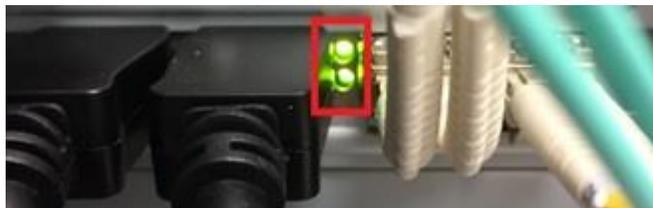
**Figure 134: LEDs on the Beamformer Control Board**
