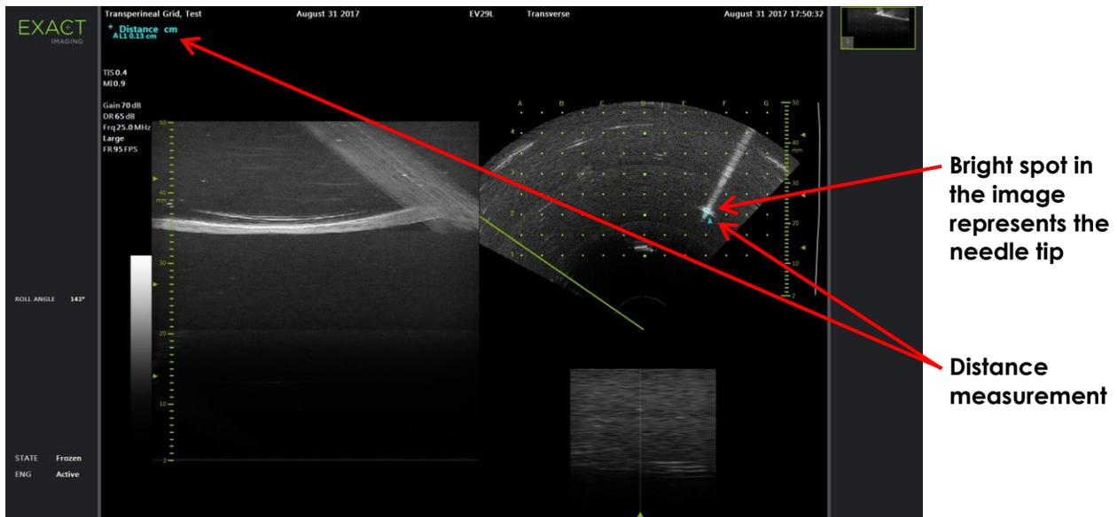
**Figure 168: Measured Distance Between Transperineal Grid and Needle in Location e2**
