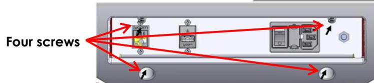
Figure 116: Screws Securing IO Plate Assembly
