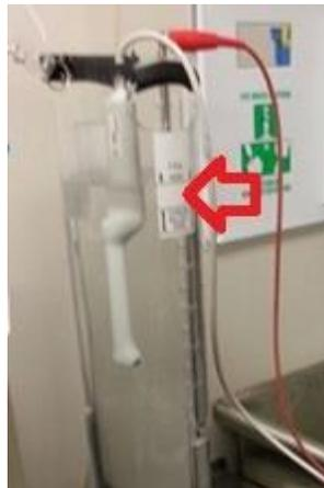
Figure 173: EV9C Transducer Immersed to its Soak Level
