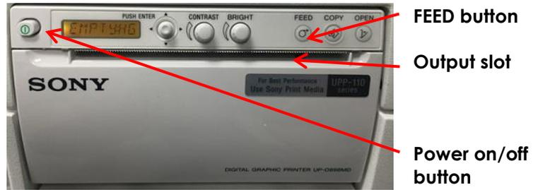
Figure 131: Printer Control Panel
