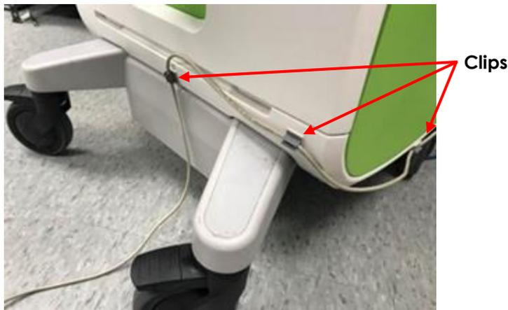
**Figure 19: Foot pedal cable clips**
