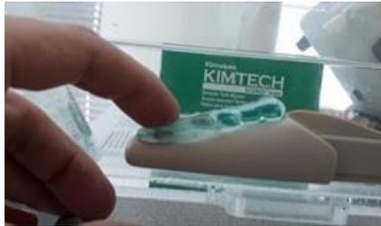
**Figure 155: Gel Applied to EV29L Transducer**
