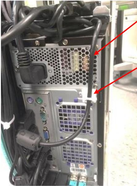
Figure 75: Routing Display Port to HDMI Adapter Cable
