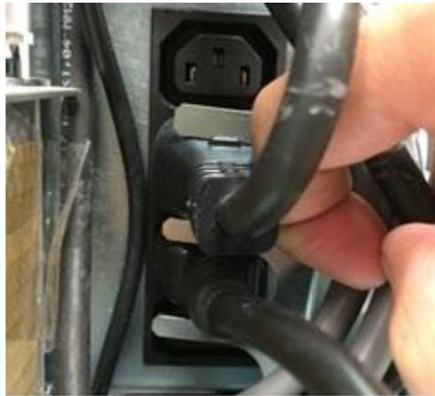
**Figure 140: Computer Unit and Control Panel Height Control Power Cables**
