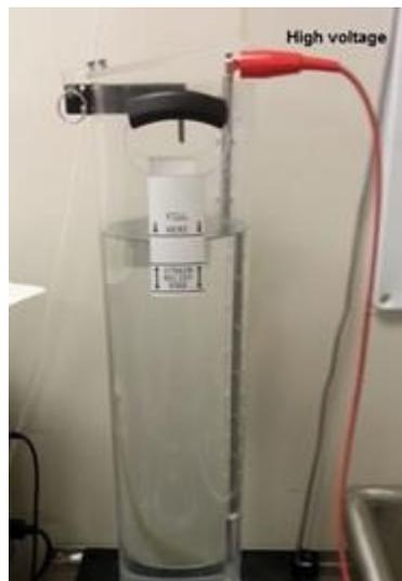
**Figure 171: Connect Safety Analyzer to Safety Test Tank**
