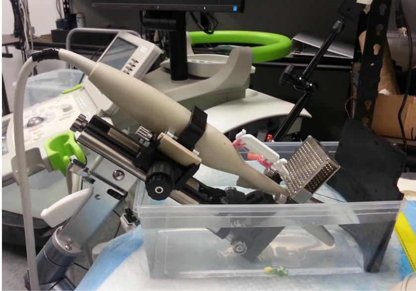
**Figure 166: Transducer and Transperineal Stepper in Water Bath**
