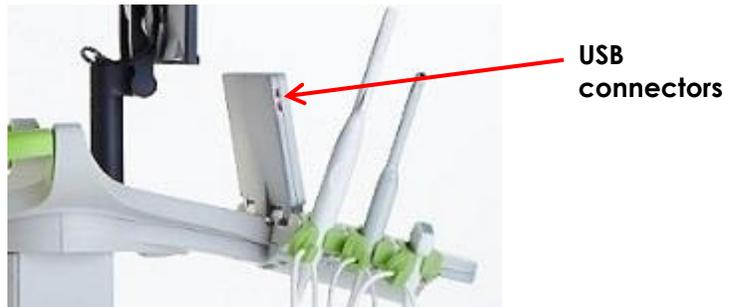
Figure 37: USB Connectors on the Left Side of the Touch Screen
