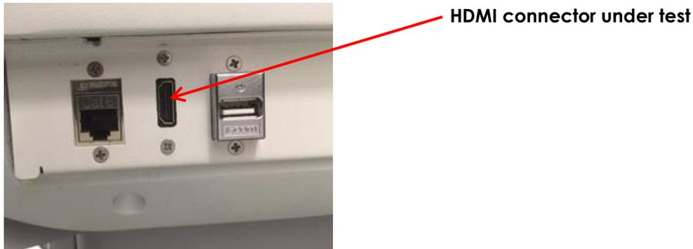
Figure 132: View of I/O panel at the back of the system
