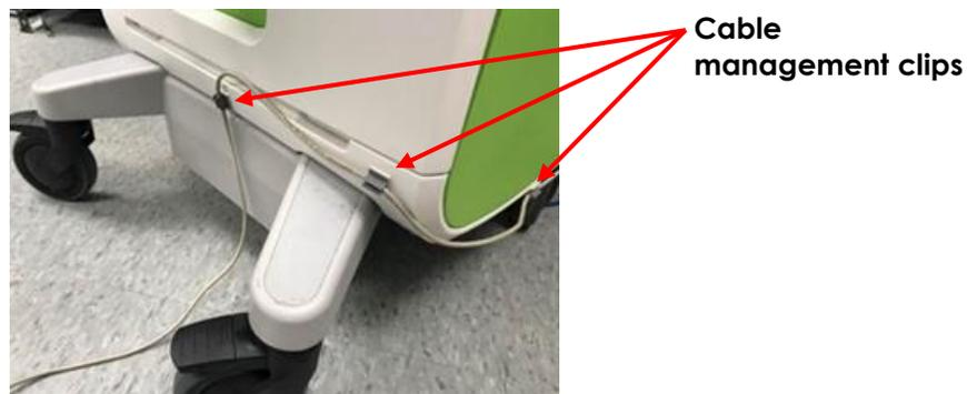
Figure 6: Foot Pedal Cable Management
