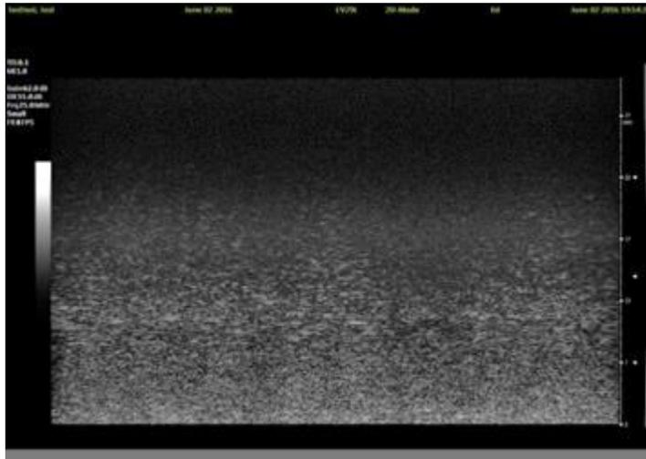
**Figure 144: 2D Mode with the EV29L Transducer and Tissue Mimicking Phantom**
